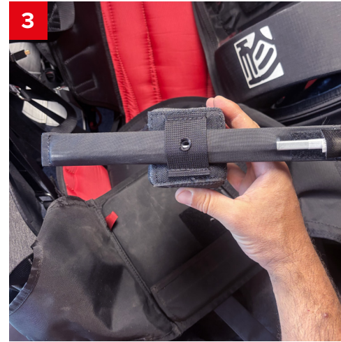
3 Introduce the paracord through the chosen footpad and the bars
