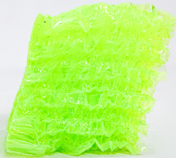
Damaged cell (Needs to be replaced)
