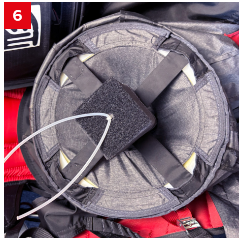
6 Make sure the 4 bars are locked into the fabric pockets
