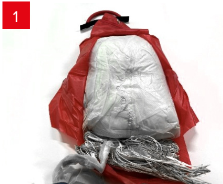
1 Place the folded rescue into the inner bag
