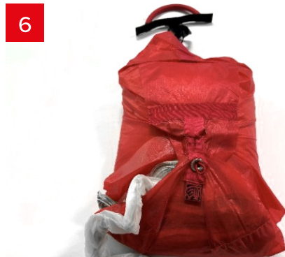
6 Cover the bottom cover, and use a central elastic band to pass through the bottom eyelet hole
