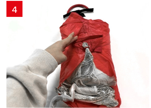
4 Secure the suspension line using the elastic band
